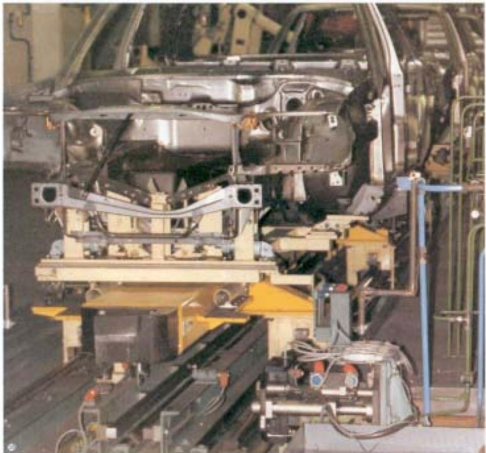
② – ③ WALTHER docking systems on different transfer lines for electricity and fluid supplies between transfer line and pallet, on welding lines and for tool changes. The electrical lines provide control as well as welding currents. The Clean Break elements mounted on the docking systems are used to seal compressed air and hydraulic lines without spillage.
