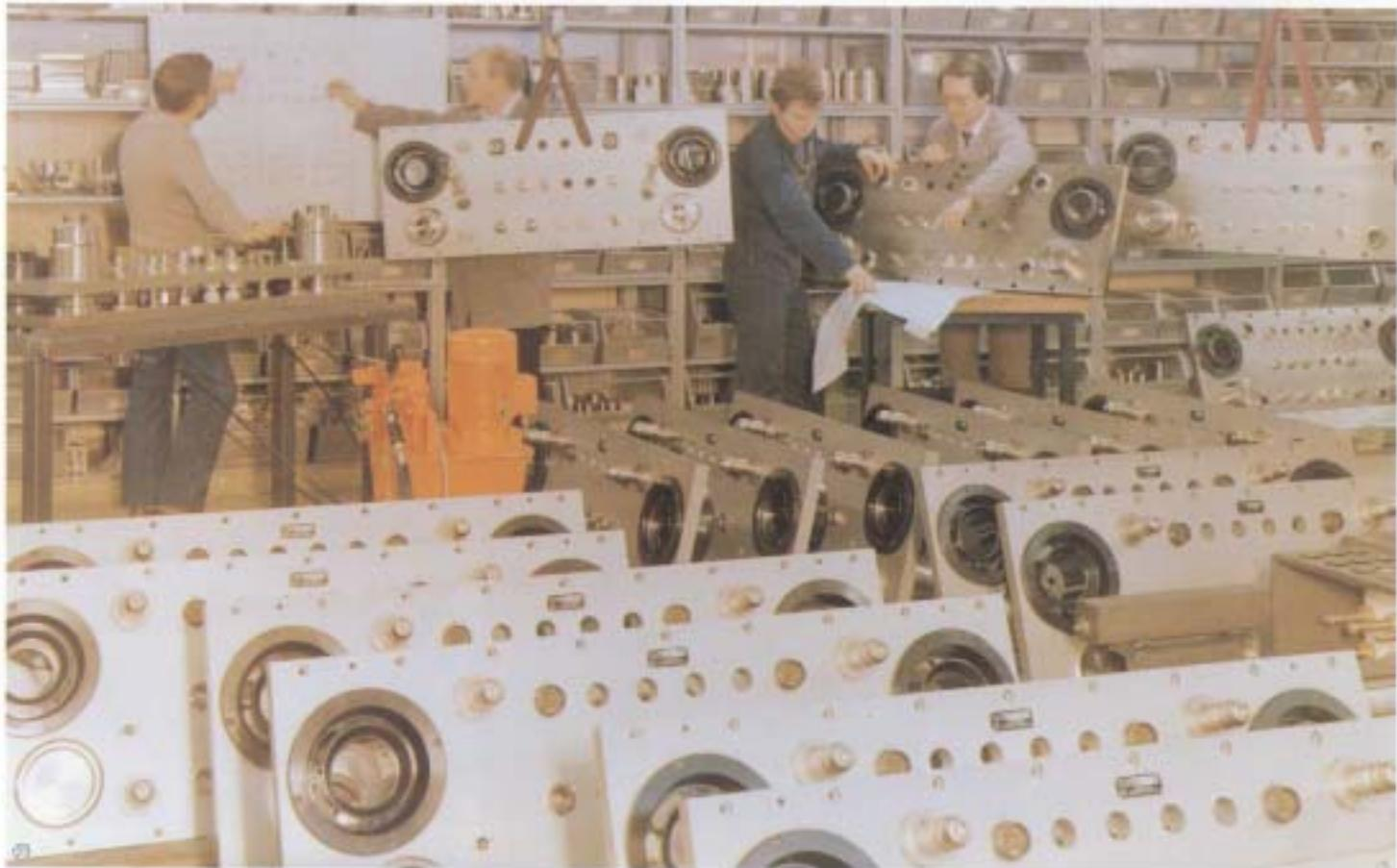
④ Fluidic multicouplings on a pressing tool.
