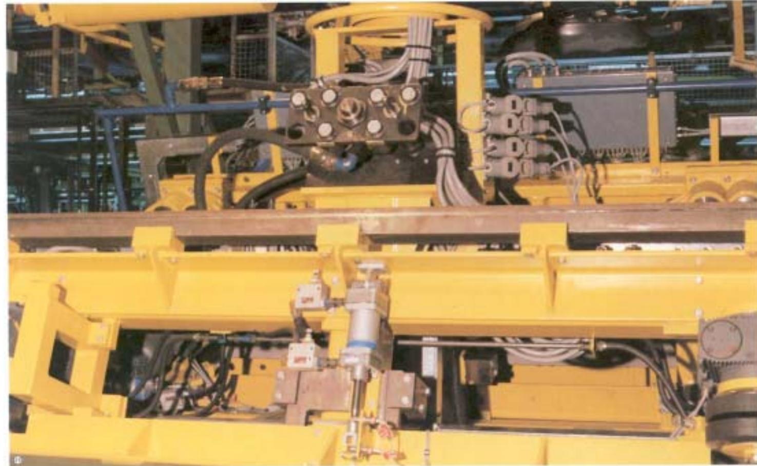
② - ③ WALTHER docking systems for automatic tool change on robots. The docking system connects control lines for welding currents, pneumatic, hydraulic and cooling water supplies. After disconnection all fluid lines seal without spillage. Connection takes place by means of a balanced force system.
