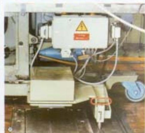
④ Manually-operated multicoupling with locking and unlocking aids for the connection of electrical and fluid lines between tool and press.
