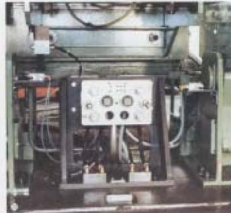
④ – ⑤ WALTHER docking system for energy supply to tool carriers in an assembly shop for securing truck wheels. Tool carriers with different multiple screw heads are located to the left and right of the assembly line in waiting areas. The energy supply lines are located parallel to the assembly line on mobile overhead gantries.
