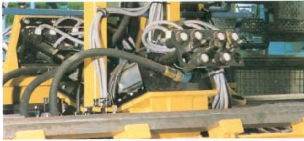
WALTHER mono- and multicouplings in a car body side line for supplying pallets with compressed air and electricity.
