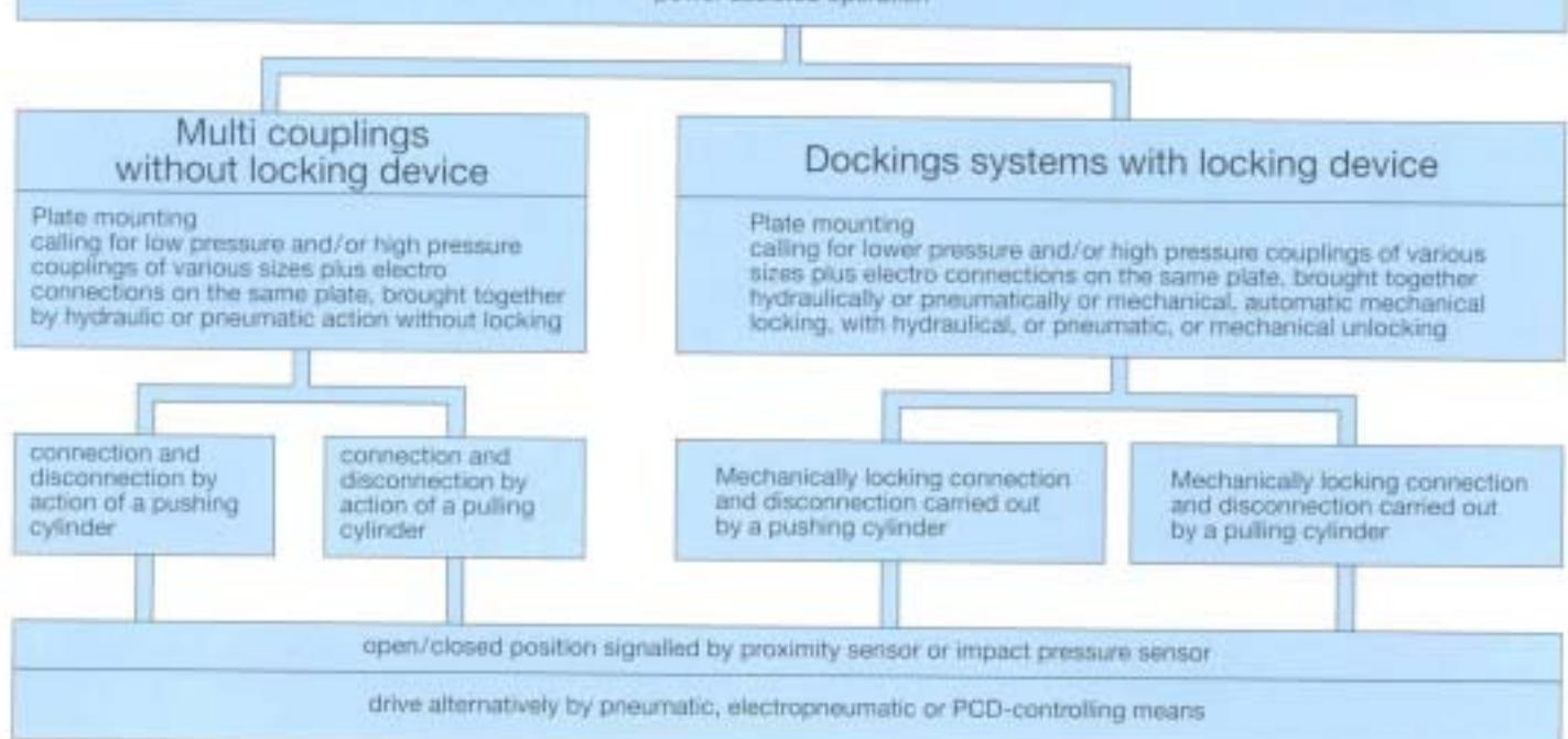
In Multicouplings and Dockingsystems one can use alternatively full flow elements, one- or both side sealing elements in standard-, high pressure-, or clean break version according to WALTHER standard sheets WWN 43.1, 46.1, 46.2, 50.1, 51.1 and 51.2.
