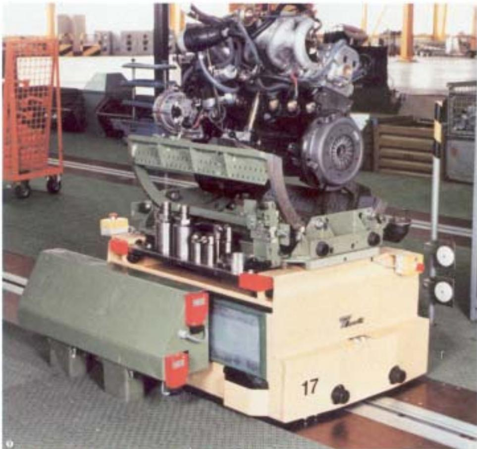
Walther docking systems have proven themselves over many years in development teststands and testbeds for the testing of Otto and diesel engines. Here the docking systems are used in vertical and in horizontal positions. The docking systems serve to connect the fluid and electrical lines between engine and teststand. Media discharge is safely avoided by having a Clean Break coupling on each medium line, thereby ensuring spillage-free disconnection.
