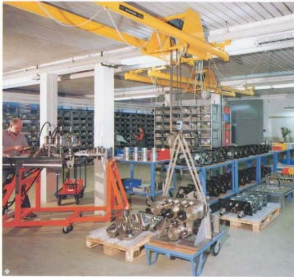
① ② Final assembly of WALTHER multi-couplings and docking systems for test stands and transfer lines.
