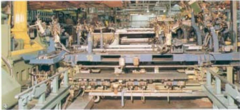
⑦ – ⑧ WALTHER docking systems for connection of pneumatic lines in transfer lines. In order not to subject the pallets to additional forces, the docking is effected by means of a balanced forces system. In this way no force is transferred to the pallet.
